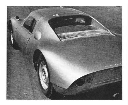
lowing room underneath for essentials such as a 29-gal. fuel tank, oil radiator, battery and spare tire. The rear of the car is chopped off sharply in the utilitarian modern manner.
